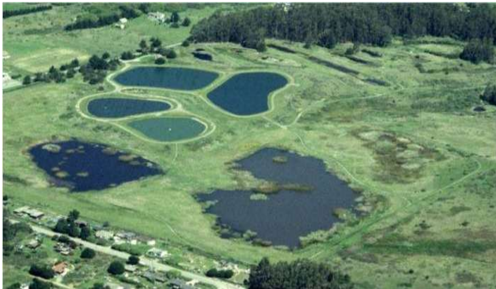
Figure 5-13. Bolinas, California AWIPS® with adjacent spray fields, including seasonal wetlands, depressions worked into the surrounding area providing habitat for birds during the rainy season. Operation rotates the area being sprayed over the dry season. Maintenance includes monitoring condition of pipes, pumps, valves and sprinklers and harvesting emergent vegetation.
